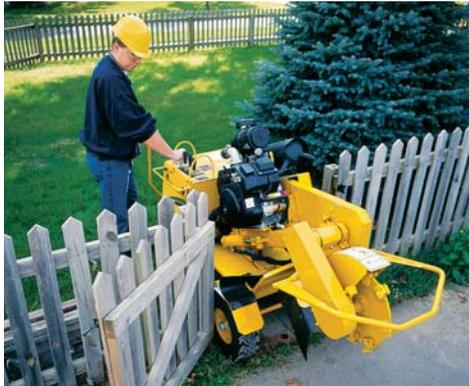
**A narrow width of 35" (88.9 cm)** allows entry through most standard gates. Additionally the SC252 is able to maneuver in tight work areas by disengaging one of the drive wheel locks.
