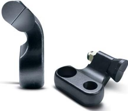
**The patent-pending Yellow Jacket Cutter System** features a universal tooth that can accommodate all cutting positions on the cutter wheel. Plus, each tooth is designed with two cutting edges. With the second edge protected from primary wear while the first edge is engaged, when the tooth becomes indexed to the second position, the opposite edge provides a like-new cutting surface for extended tooth life.
