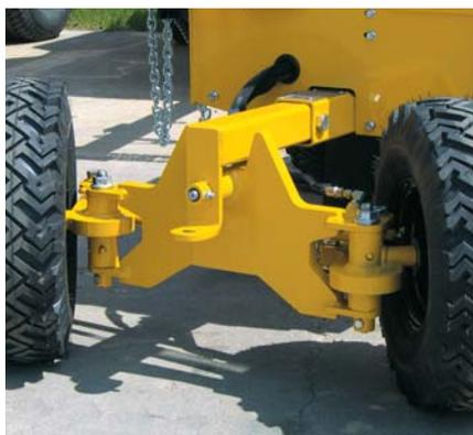
**The SC252 optional hydraulic front steer** features an oscillating axle for mobility, specially designed steering for tighter turns, an easily accessible single-lever control, and hardened steel pivot pins and bushings.
