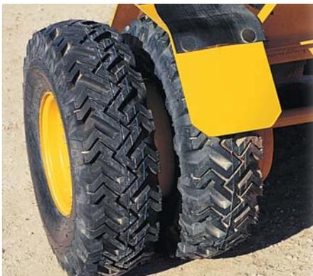
**Optional rear dual tires** improve flotation, traction and stability, enabling the operator to work more effectively on uneven terrain.
